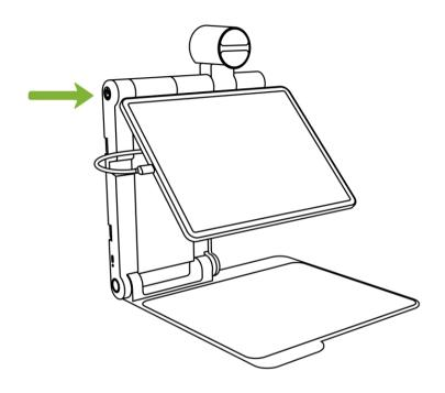
Long press the power button for 2s to turn on/ off the device and when the device is turned on, the button light is green.
