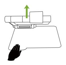
Press down on the base protrusion, and unfold the device upwards.
