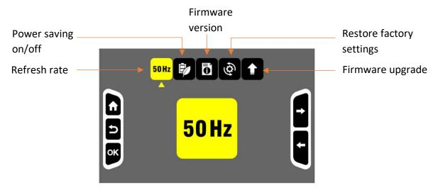
After entering the System Settings page, press Zoom in or Zoom out buttons to select the icon, press Mode button to confirm and enter the next level.
