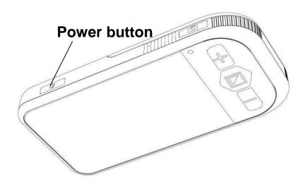
Press and hold the Power button for 2 seconds to turn the unit off. The green indicator light will turn off at the same time.
