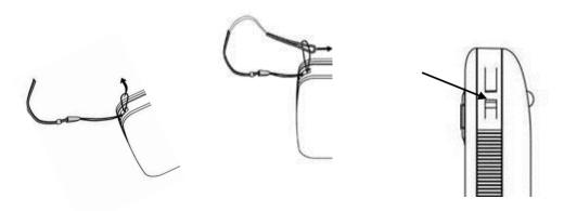
Insert the small loop through the corner of the Zoomax designed for the wrist strap. Pull the other end of the strap
