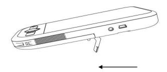
Open the Writing stand to allow you to write underneath the camera easily.
