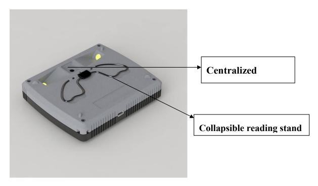
**Camera:** Butterfly features an auto-focus camera that centralizes on the screen for an optimal ease of use while reading or writing
